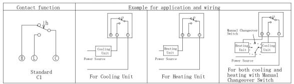
Arrow marking indicates a direction of switch action.
