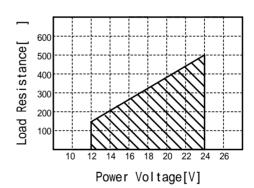
When Measuring Equipment is voltage input, connect ONE Equivalent a resistance(small temp. coefficient type) in serial as shown right figure and measures voltage drop across the resistance. (Brown) mmeasuring equipment In case of using with ONE Controller, MAX. load resistance should (Blue) be 400(MAX. load resistance (500 R 7/// GND -internal resistance of ONE(100 )). Voltage )4 to 20 mA will correspond to 1-5V at R=250
