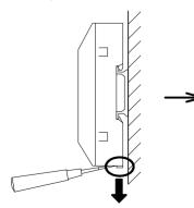
Insert a flathead screwdriver into into the hole of the fixture at the bottom of the main unit and move the fixture downward.
