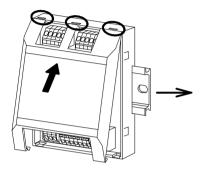
Insert the claws at the top of the cover into the grooves (3 places) at the top of the main unit.
